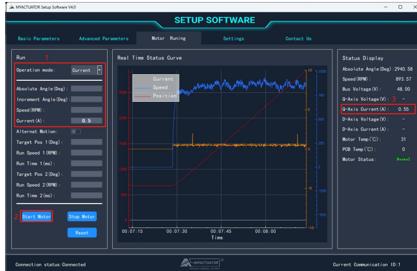
Figure 4-5 Schematic diagram of current mode operation
