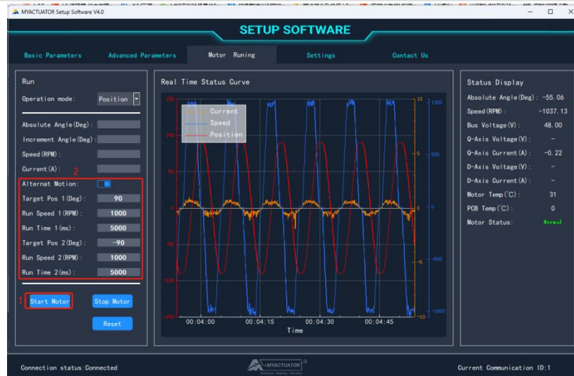
Figure 4-6 Schematic diagram of alternate motion mode operation
