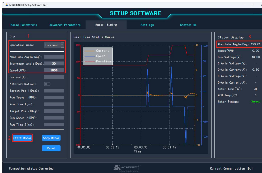
Figure 4-3 Schematic diagram of incremental mode operation
